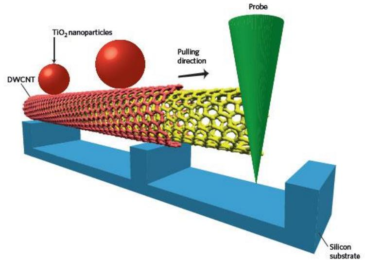
Macroscale superlubricity enabled by graphene nanoscroll formation
